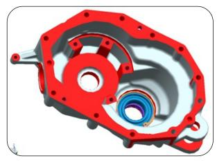
33. Press the ball bearing 6209 on rear axle house LH/RH Put circlip to lock the bearing in rear axle housing LH/RH
