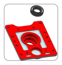
51. Assemble seal in PTO retainer as shown.
