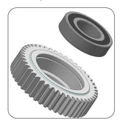
46. Place the gear driven (Z- 49/ Z-51) on fixture. Put the bearing on ram
