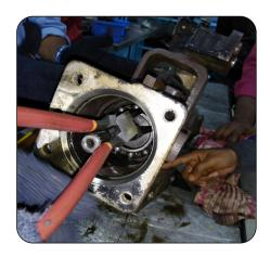
Remove spacer of 3mm. Remove shims.
