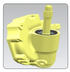
• Press sleeve oil seal on knuckle housing.
