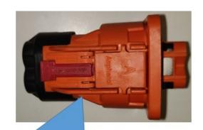
Push the Connector to mating part to fully close the same. Ensure that Lock / unlock lever is in Unlock position and connector is assembled in right direction as per snapshot
