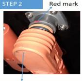
Match this arrow mark with the centre of red mark shown above and push the connector inside the mating part such that it fits in it
