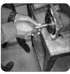
• In Differential assy, left hand shaft is smaller than right hand.
