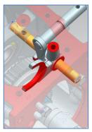
59. Lock the position of fork shifter in rail with steel ball, spring and screw grub in fork.
