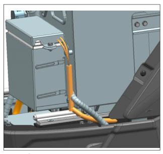
Step 5 – Disconnect Auxilary Battery Connector
