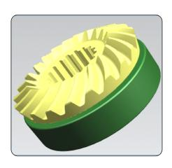
Assemble the crown wheel with the ball bearing 6210. Assemble the crown wheel and bearing sub-assy on differential case splines.
