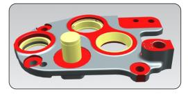
14. Put the intermediate plate on fixturePress 4WD pin in platePress bearing 30205 outer race.Press Bearing NJ205 outer race in plate.Lock NJ205 outer race with circlip.
