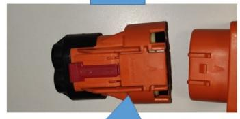
Pull the connector outside to dismantle completely
