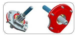
36. Assemble bull pinion shaft LH/RH with bearing & lock it with circlip Assemble bull pinion shaft assembly in brake housing LH/RH & lock with washer & Screw.
