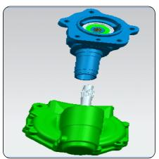
Press taper roller bearing outer race 30304 in cover knuckle.
