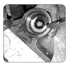
• Open 4 bolts M8 allen & Use two jumping bolt to open
