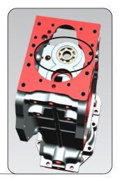
5. Put the bearing in the CH housing from opposite side as show in pic.
