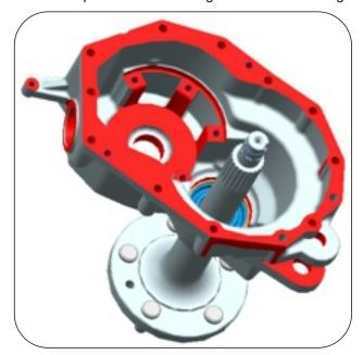
34. Assemble axle shaft LH/RH as shown assembly with bolt in rear axle shaft.
