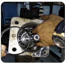
Use drift shaft & hammer to hit the differential assembly to take out whole assembly from right hand side.
