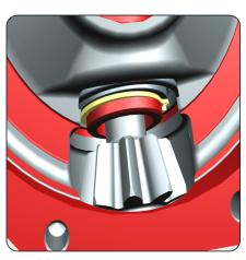
After pre loading set the backlash of gear driver bevel Z-10 by putting shims between bearing 6206 and circlip.
