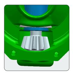
• Tight the cover with bolt M8 4 nos. And torque at 20-25 NM.
