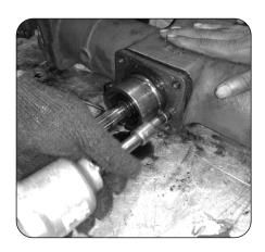
• Separate the Retainer & bevel pinion Shaft Assy.
