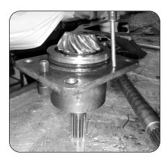
• Place the pinion shaft on fixture
