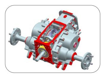
68. Assemble shaft input TO (Z 13/11) in center housing top bore from rear side.
